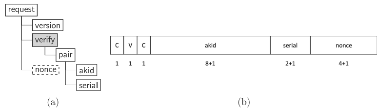
Fig. 5. The CBOR-encoded data structure of an TinyOCSP request. (a) Gray boxes indicate an array containing any number of duplicates of its nested contents. Dashed boxes are optional to include. (b) Shown as message payload in bytes, for querying the status of one certificate, including an optional nonce and CBOR headers.
